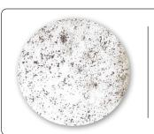
Standard plastic pan with visible mold
