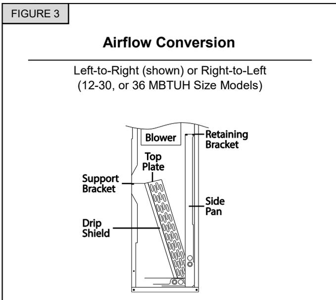
6. Remove the screws holding the coil bracket to the left side of top plate. Reposition coil support bracket to right side of top plate.
