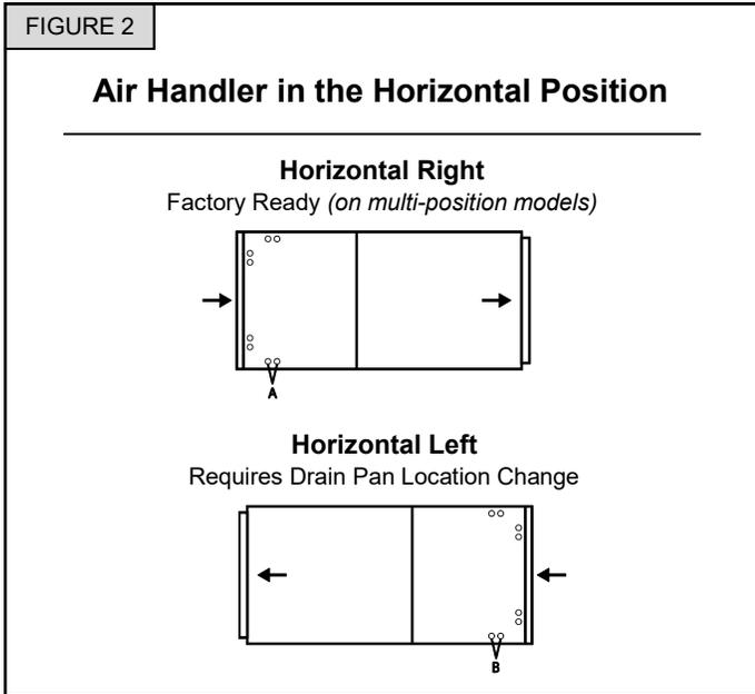
Models listed in Figure 3 are shipped in the horizontal right airflow configuration. To convert to horizontal left airflow, follow these steps:
