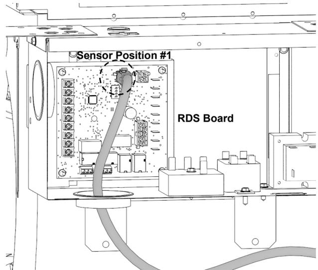
**NOTE:** F-series air handler will be factory configured for the up flow application with the A2L (R-454B & R-32) refrigerant sensor positioned at the bottom of the air handler as shown.
