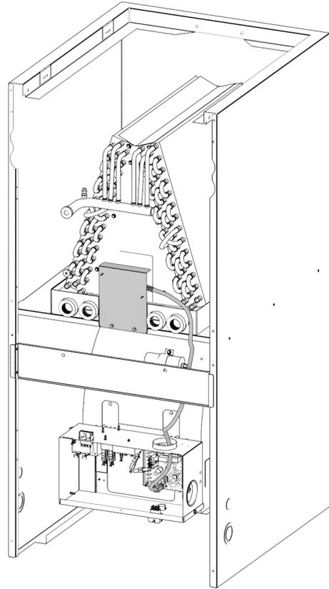
6. Ensure that the sensor is mounted so that the sensing element is facing the coil and it is not blocked by the distributor tubes or the TXV.
