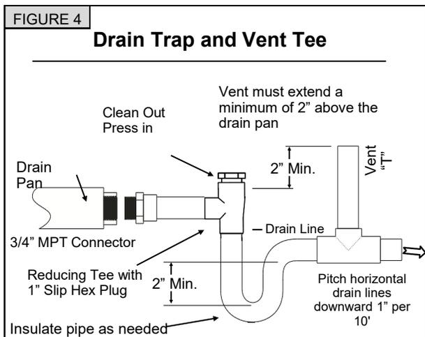
Route drain line so that it does not interfere with accessibility to the coil, air handling system or filter and will not be exposed to freezing temperatures.
