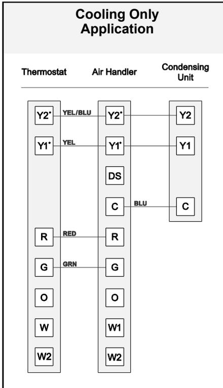
For typical 2-stage operation, move motor tap 3 (YEL) to Y2, and move motor tap 2 (BRN) to Y1.
