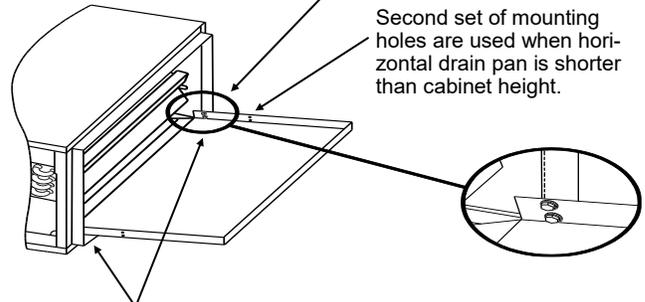
Second set of mounting holes are used when horizontal drain pan is shorter than cabinet height.
