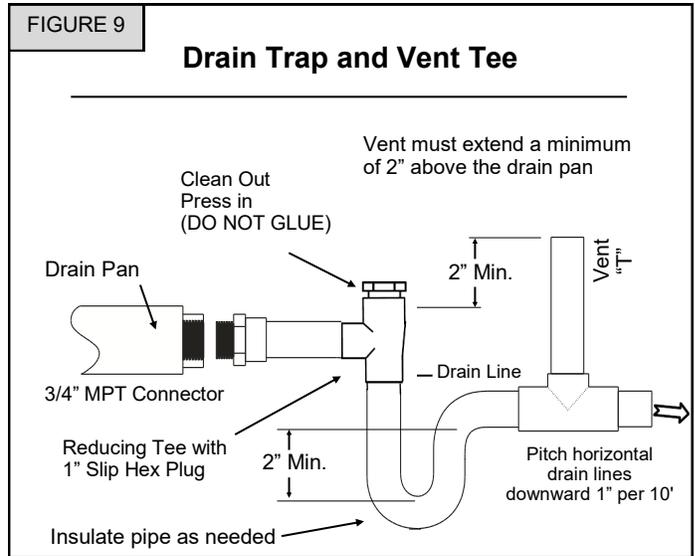
flow with unit in operation. An auxiliary drain pan should be installed under the unit, and have a larger footprint than the coil, as specified by most local building codes.
